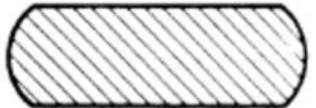
No. 4 Edge (round) Rounded corners – may be flat with slitting fracture visible across the edge
